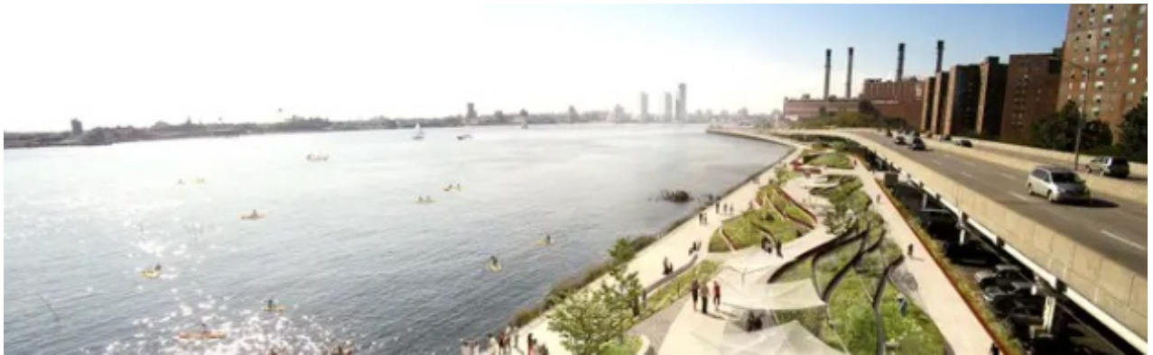
Below: New York's Big U project. Coastline open spaces designed to accommodate floodwater during storms and/or as a result of sea level rise.
