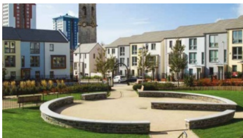
Above right: Basketball and skateboarding facilities incorporated into public realm that feature seating while functioning as flood water collection pools in rainstorm conditions.
